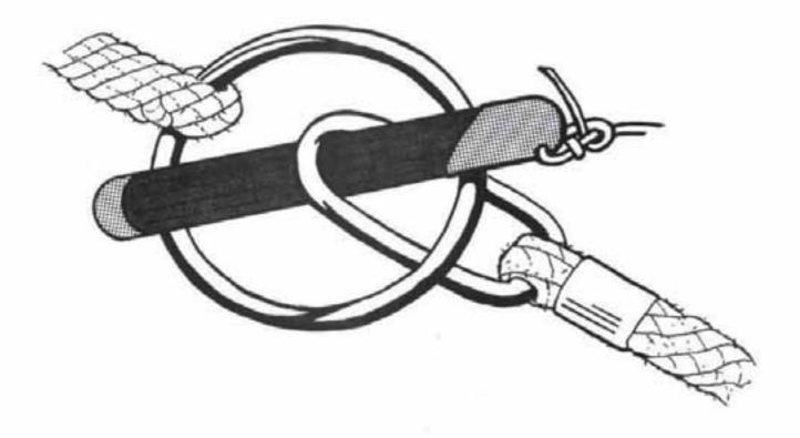
Figure 2. Manual release pull-pin mechanism for dropnet.
